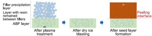
Fig.11. Adhesion improvement mechanism by dry ice blasting filler removal
