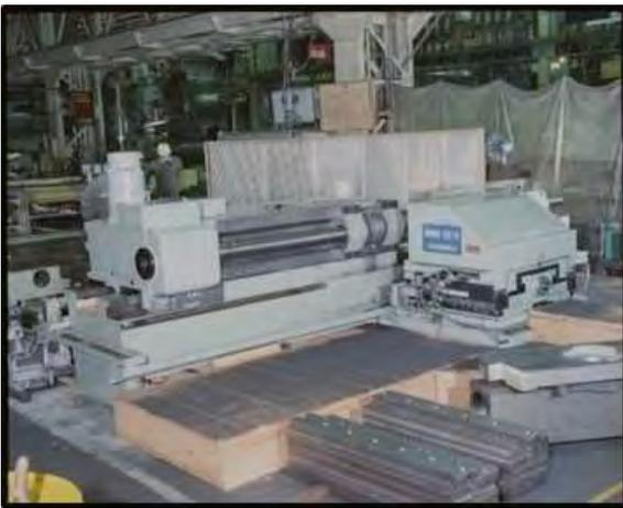
**Fig.18.** The machine dedicated to worm & rack and nut processing MWR-3510
