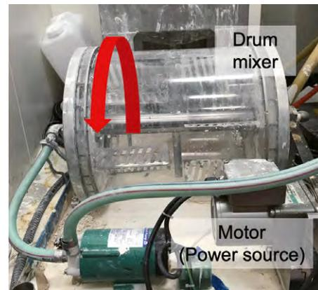
Fig. 9. Electrically driven rotating tank.
