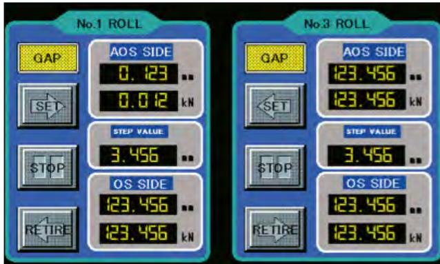
Fig.7. Operation screen of hydraulic servo system
