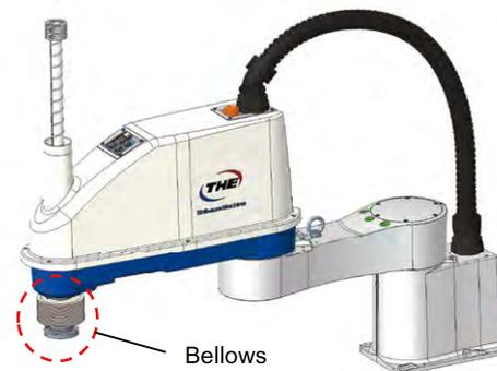
Fig.3. Outer appearance of THE800 (bellows specification)
