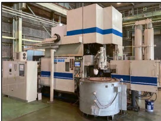
**Fig.2** Die-casting machine with a clamping force of 3500 kN (servo oil as pressure source, with intensification accumulator)
