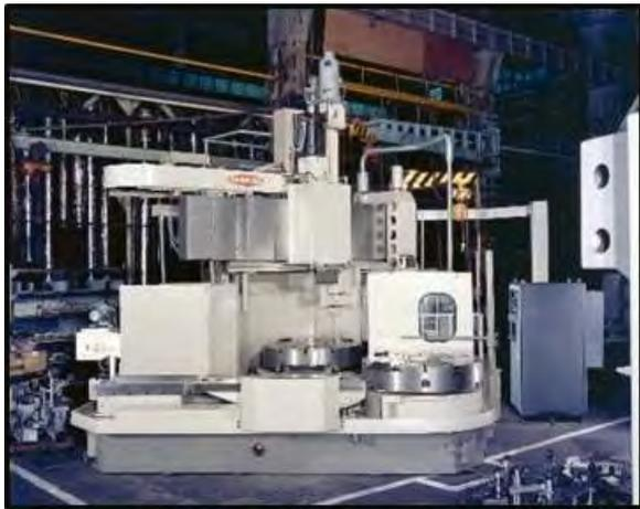
**Fig.20.** NC vertical lathe TMC-13A (with automatic pallet replacement function)
