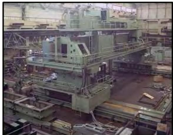
Fig.17. Gantry type NC Plano Miller MG-24/14A
