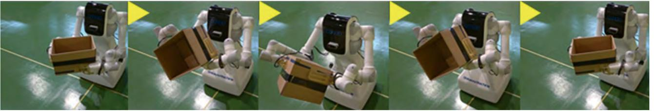
**Fig.8.** Tipping over a cardboard box by an actual CONOID-III robot
