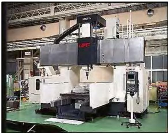
Fig.23. MPF-C series double-column machining center
