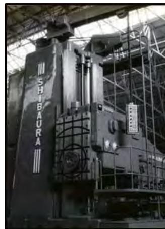
Fig.11. Large horizontal boring machine
