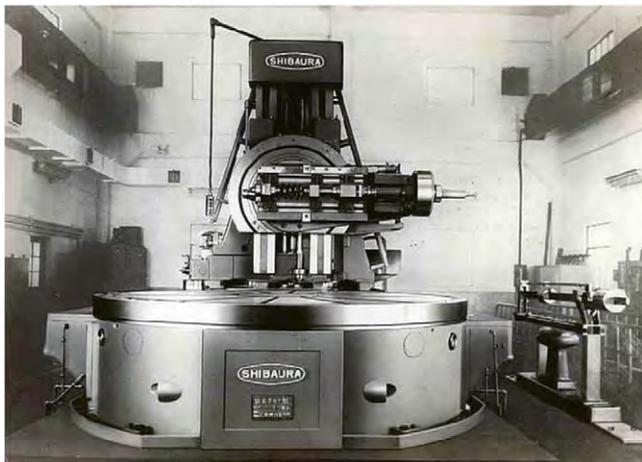
Fig.9. Master gear hobbing machine HRS-500
