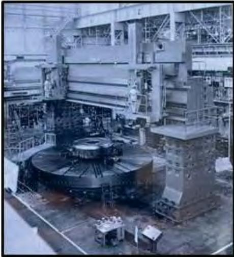
**Fig.14.** Large vertical lathe TWI-80/120
