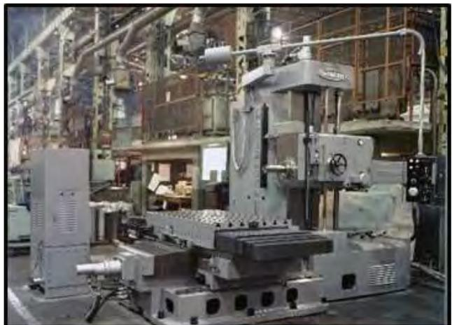
**Fig.13.** Table-type horizontal boring milling machine BFT-9(S)NC
