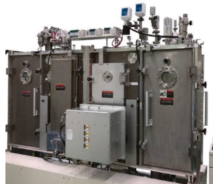
Fig. 3 Sputtering system for reforming using plasma treatment
