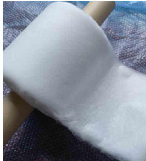
Fig. 15 Meltblown nonwoven fabric sheet which was made of degraded PP by high shear extruder. We used PP2 as the raw material because no talc was included as the additives.
