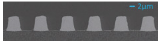
Fig. 14 Cross-sectional SEM image of the " LS = 5/5 \mu\text{m} " section
