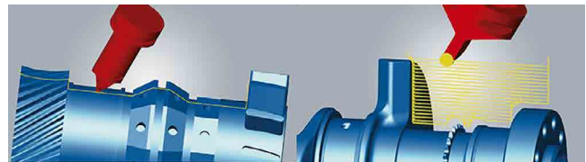
Fig. 3 Simultaneous 3-Axis Turning
