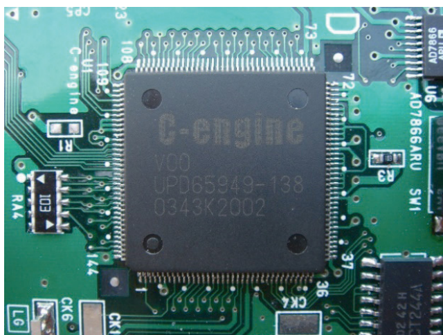
Fig. 11 Developed current control LSI C-engine
