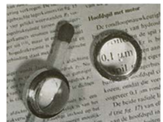
(c) Plastic lens formed by ultra-precision mold
