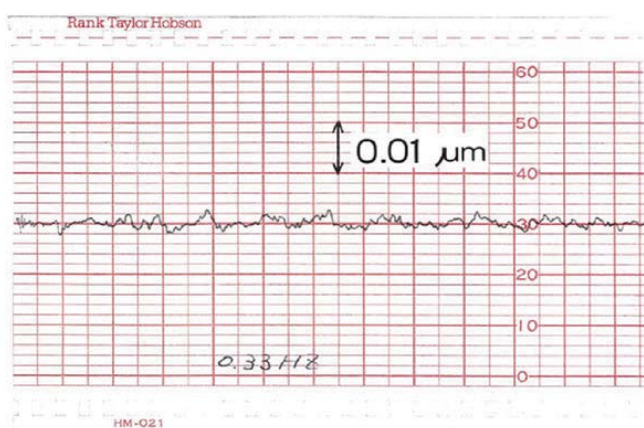
Fig. 14 Surface roughness of polygonal mirror machined by fly cutting
