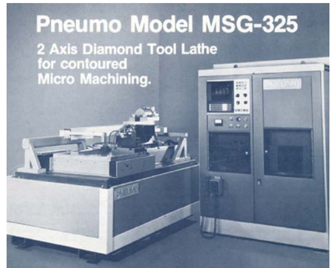
Machine configuration and accuracy (1) Aerostatic spindle: Runout accuracy = 0.1 \mu\text{m} (2) Aerostatic guideway (3) Control resolution: 25 nm
