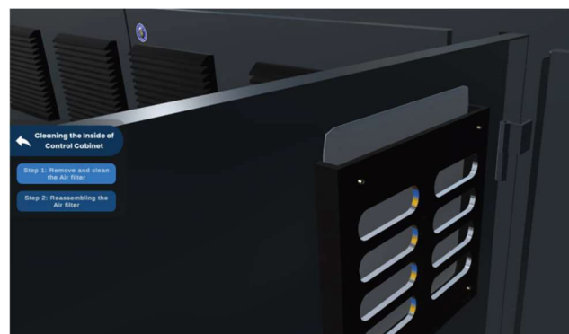
Fig. 16 Control cabinet air filter cleaning
