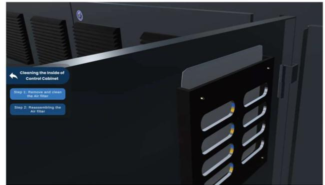
Fig. 16 Control cabinet air filter cleaning
