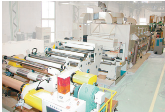
二軸延伸フィルムテスト装置 Bi-axial oriented film manufacturing equipment to develop process
