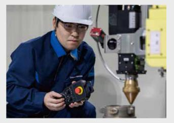
金属3D積層造形装置 3-D Metal Additive Manufacturing Equipment
