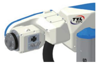
Wiring and piping to the robot tip can be connected through the inside of the robot Prevent wires and air tubes from getting tangled by changing the position of the connection panel.
