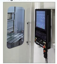
Improved operability and visibility achieved with the operation panel that can rotate from 0 to 90 degrees and the diagonal door.
