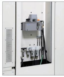
Easy maintenance achieved by placing the devices that require daily inspection together on the back panel of the machine.
