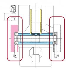
The chip conveyor and the coolant unit can be installed on either the left or the right depending on the layout. (Supported as an option)
