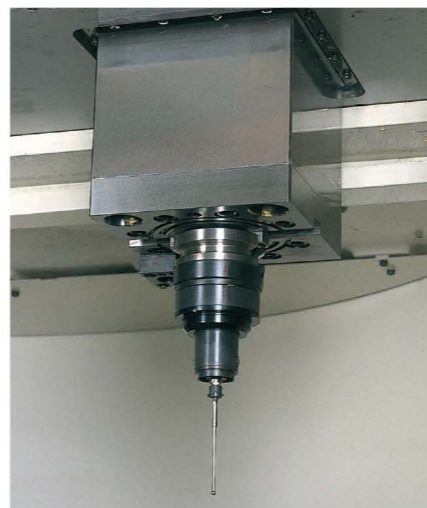
10 Automatic diameter and step difference measuring device
