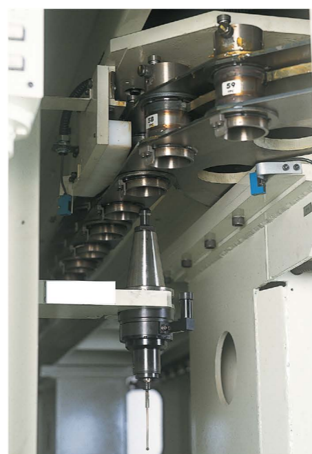
2 Automatic tool changer (ATC) Photo shows for ATC 48/60 tools
