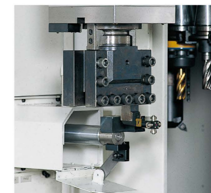
11 Automatic tool tip measuring device
