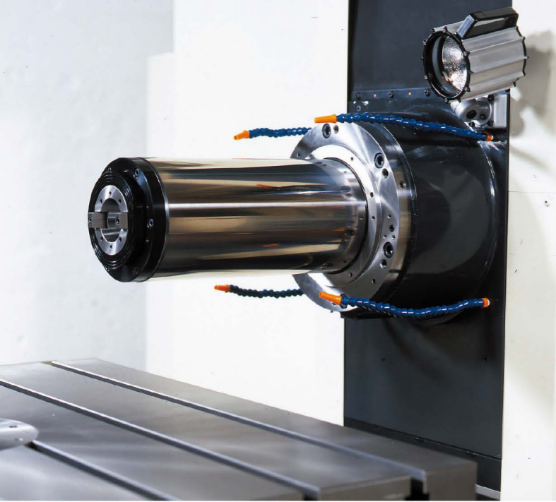
Quill at 400 mm extended (W-axis)
