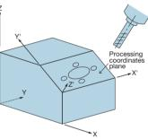
simplify machining of an inclined surface without effort.
