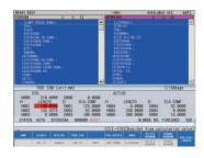
upon machining. These three screens run independently during automatic operation and during editing
