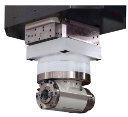
Maximum power : 3kW at 100 min<sup>-1</sup> Maximum torque : 286N·m(29kgf·m) Maximum speed : 2 000min<sup>-1</sup> **Tool change : AATC** (An optional special tool changer with AATC feature is required) Allow AAI : at every 90 positions
