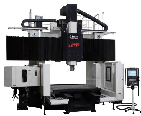
There is a sister seires of MPF-F on which crossrail is fixed and has no elevation movement.
