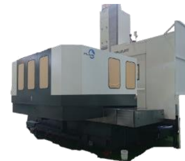
Large-scale horizontal boring and milling machine for milling gearbox for offshore wind turbines
