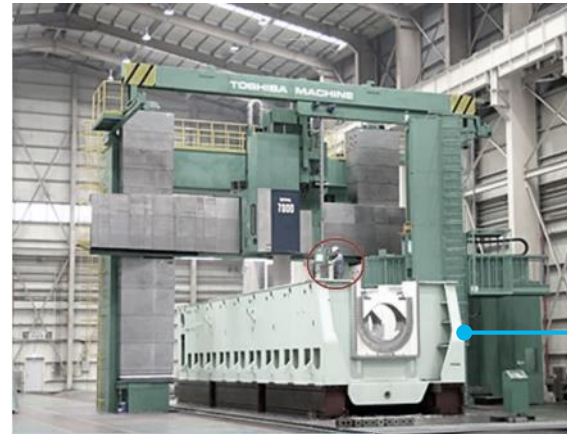
Ultra-large-scale machine tool for milling for tanker engine block transporting oil and gas
